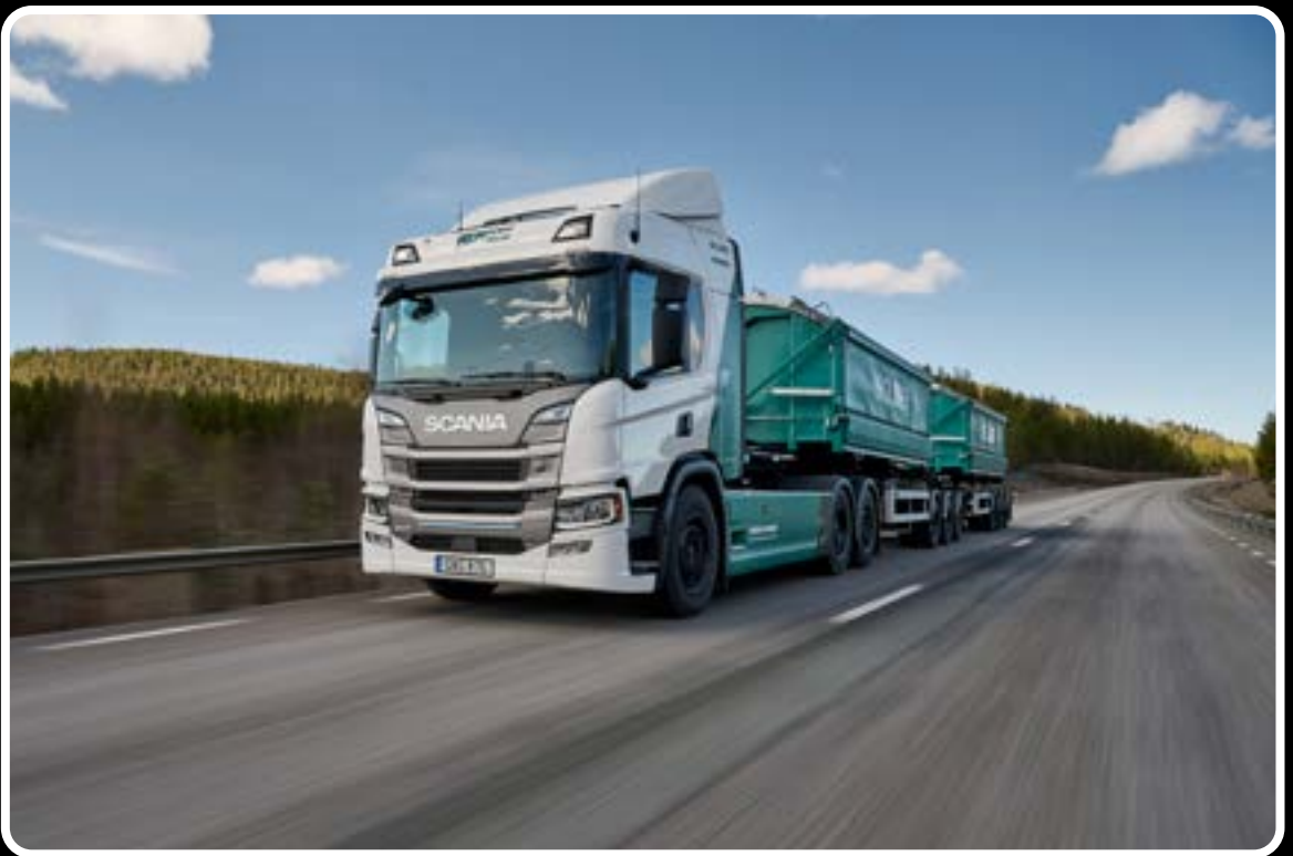
As of 2023, Scania's biggest truck is the model 770 S. With a 16-litre engine of 770 hp, the truck's train can bear 77 tonnes of approved gross trailer weight. (Photo: Dan Boman, Scania)
