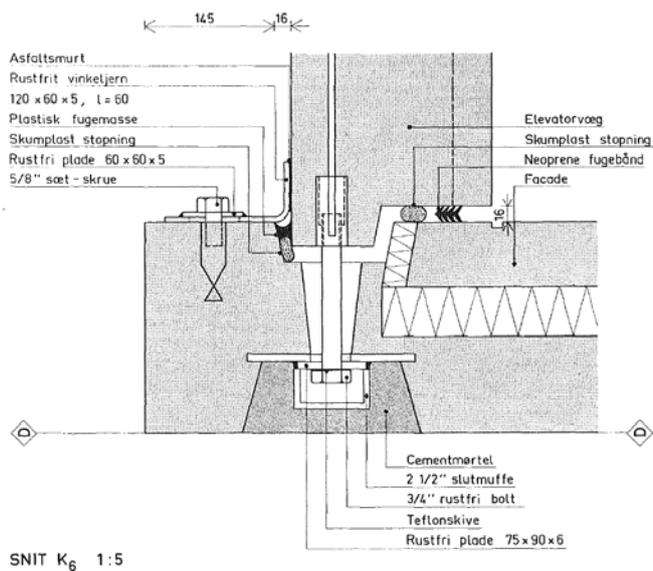
*Horizontal section in joint between facade and exterior elevator tower in the LN-BO system. Many parts had to be mounted accurately to avoid later construction damage. Poorly instructed unskilled workers and failing control was the weakness of industrialized construction (Nissen 1984, p. 301).*
