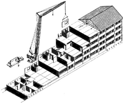
*The over 400 m long Vesterbo building in Værløse created an international breakthrough for LN in 1959. Many countries were impressed by the LN-BO system, including the delivery of elements with everything mounted (Nissen 1984, p. 283).*
