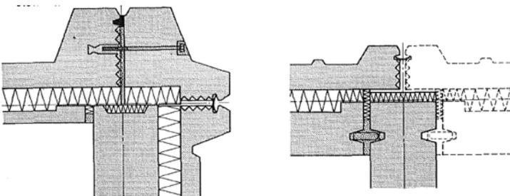
*The assembly of elements was continually improved. On the left is an assembly of a corner from the Hareskovvej building in 1958; on the right is an assembly from Bellmansgade from 1962 (Nissen 1984, p. 47).*
