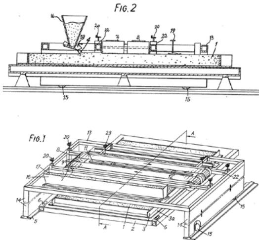
Patents were essential to LN for the company to maintain its position as one of the world's leading suppliers of finished element foundries. This casting machine for smooth slabs was patented in 1971 (patent GB1402317A).
