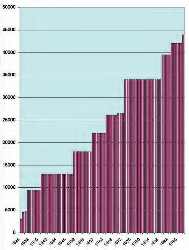
The figure shows the load for the heaviest truck delivered from the Volvo factories. From each model is taken the heaviest combination of truck and trailer. The data behind the figure is not so accurate that it is possible to know the year of the heaviest truck; generally the year of the first appearance of a model is taken. As seen the capacity is moving upwards rather stable. Volvo is a typical manufacturer of heavy trucks. The general picture will be rather similar.
