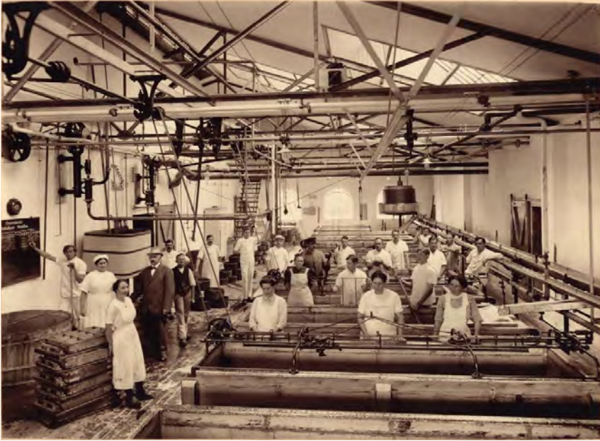
Cheese vats in rows in Denmark's largest cooperative dairy Trifolium in 1915. Still, the stirring was carried out in the large vats with a cheese grip. At that time, few dairies produced cheese, and if they did, they rarely had more than one cheese vat. The Labor Movement Library and Archives, picture 33.
