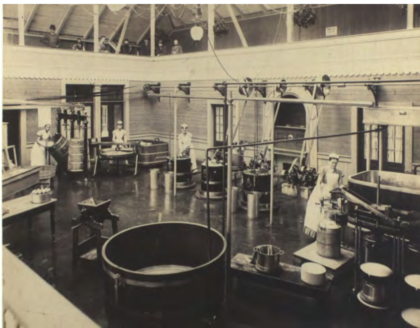
The ideal for a modern dairy in 1888 with machine-driven centrifuges and beginning piping of milk was set up at the Nordic Agricultural and Art Exhibition in Copenhagen. To the right is a cheese vessel and in the foreground filled cheese molds. Photo Juncker-Jensen, Royal Library DT023141.
